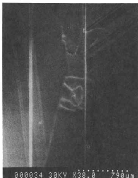
Figure 7: Thermal-wave image of Si solar cell material showing grain structure.
